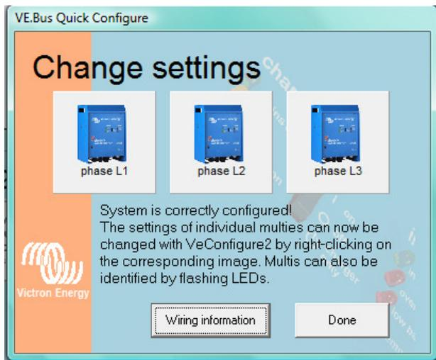
You can start VE Configure by using your right-click mouse button while you are hovering over a unit with your mouse pointer. In this same menu, which will pop up, you can also choose the [Flash LED's] option. The LED's start blinking on the corresponding unit and you can check if the AC wiring is correct.
