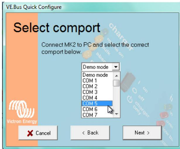
In order for the computer to find the converter, the correct port number should be selected. See page 2 of this manual to find out how you can find the correct Com port number.
