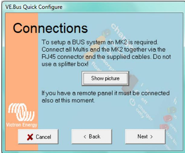
For a reliable operation of the VE Bus System it is of the utmost importance that all wiring is connected properly!
