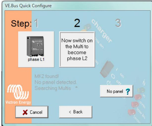
Follow the instructions on the screen and switch on all units one by one. Then wait for the program to detect the unit. When all units are detected and setup by the program, their color changes from grey to blue.
