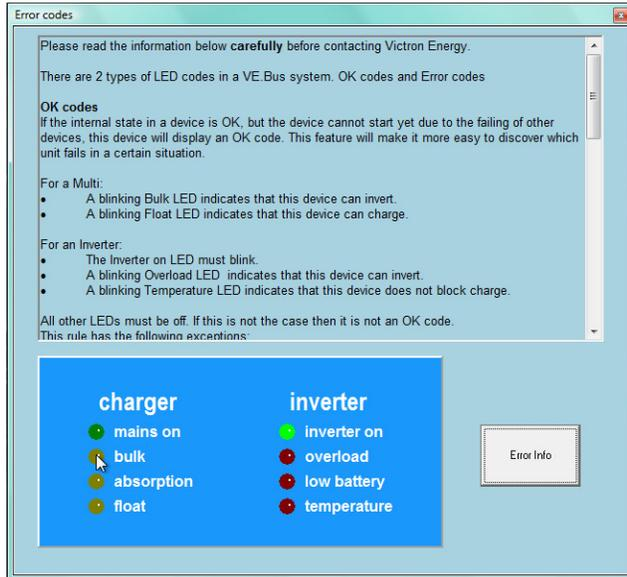
With the mouse you can make the LED's on the left side illuminate and/or blink; identical to the LED's on the real unit.
