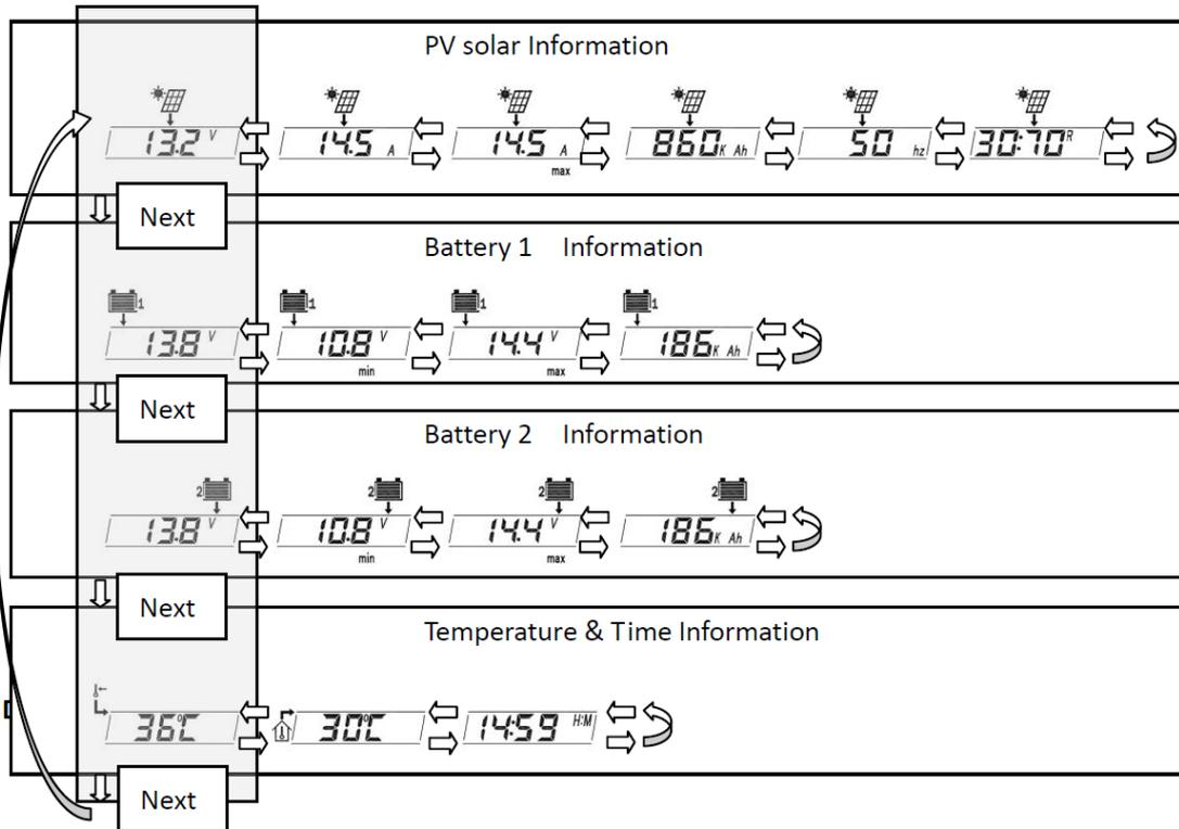
**Data setting instructions:** on reading display, press K4 for setting and next data, then save it. K1 for next data, without save. K2 and K3 to modify the data, shows as following picture.
