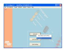
Step 3: After selected "load settings" simply choose the vsd file which should be uploaded in the Victron unit.
