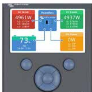
Color Control GX, showing a PV application
